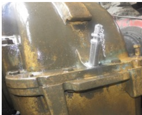
Dipstick sample unit installed on a large gearbox
