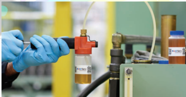
A vacuum pump sampler in use
