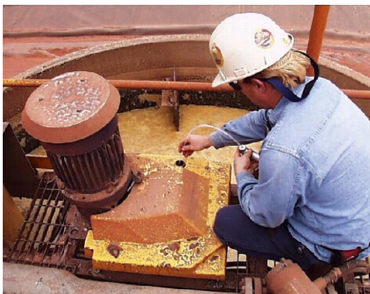
Insert tube into sample access point
