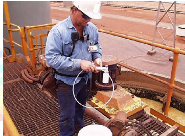
Insert a clean sampling tube and bottle
